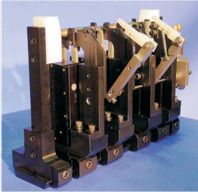
This fixture accepts two parts that are ground simultaneously. Each part is 90mm/3.50" long with diameters of 12.2mm/.50".
