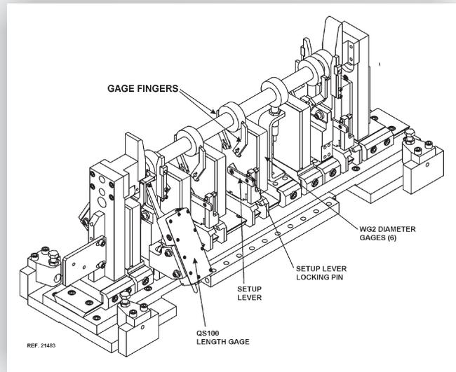
Drawing above is representative of dozens of camshaft gage stations built with this modular design concept.
