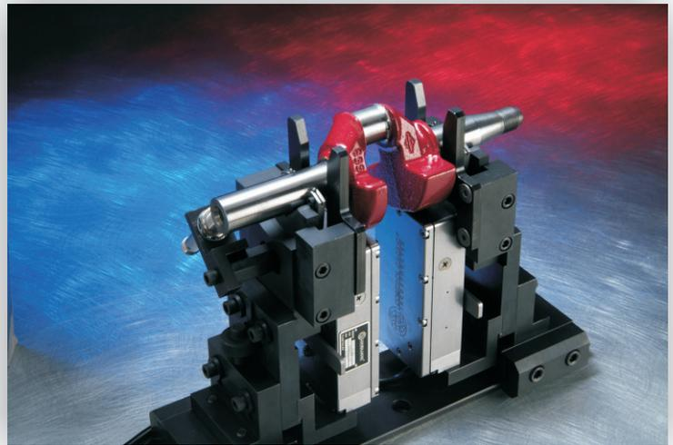
This fixture for small crankshafts measures two diameters from 22.2-25.4mm (.88-1.0”) and lengths from 200-300mm (8-12”).
