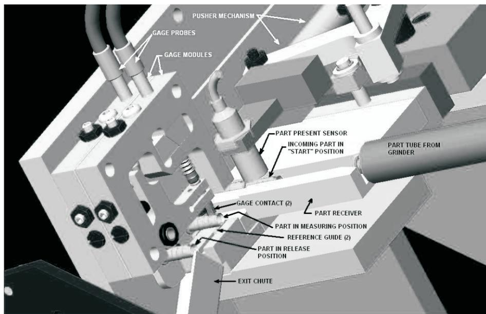
Gaging parts dynamically reduces mechanism, cuts measuring time
